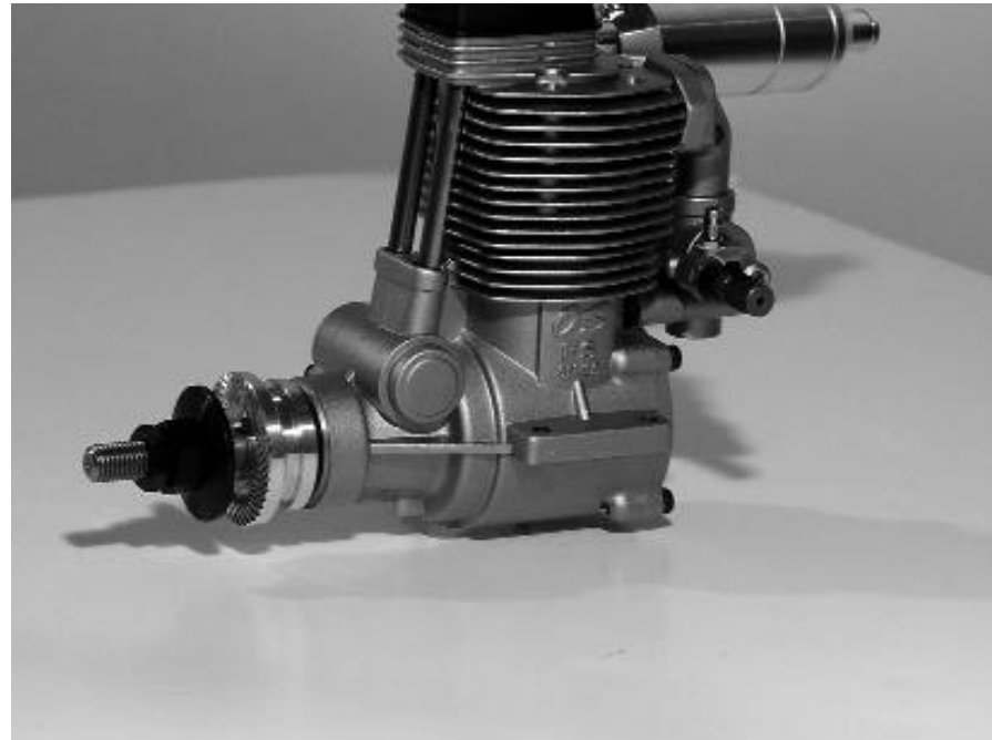
Vic used the O.S. .91 FS II Surpass (above) and found it was plenty of power, and fit nicely in the cowl. No adjustment was needed to provide a smooth transition from low to high throttle. A combination of different Futaba servos (below) and receiver (R168DF) was used to guide this model.
