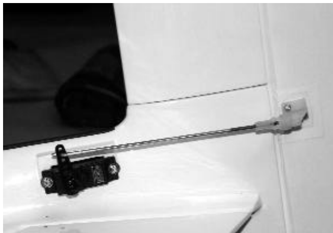
The water rudder installation. The geometry of this assembly will give you almost twice as much water rudder steering as air rudder steering. Again, much work was done to come up with this combo and it works! Don't change a thing!
