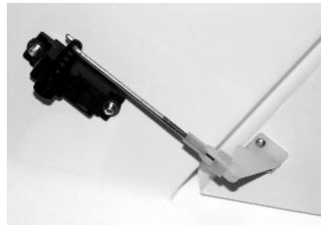
The water rudder installation. The geometry of this assembly will give you almost twice as much water rudder steering as air rudder steering. Again, much work was done to come up with this combo and it works! Don't change a thing!
